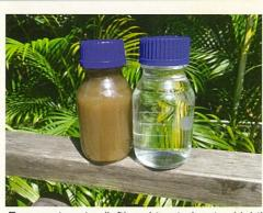
Raw wastewater (left) and treated water (right)
