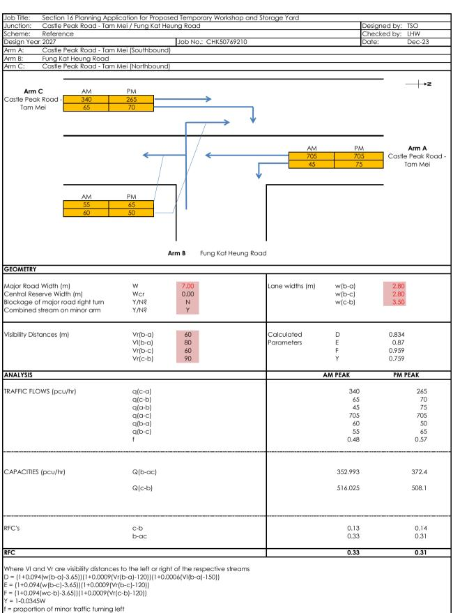
Q(b-ac) = Q(b-c)\*Q(b-a)/(1-f)\*Q(b-c)+f\*Q(b-a) Capacity of combined streams
