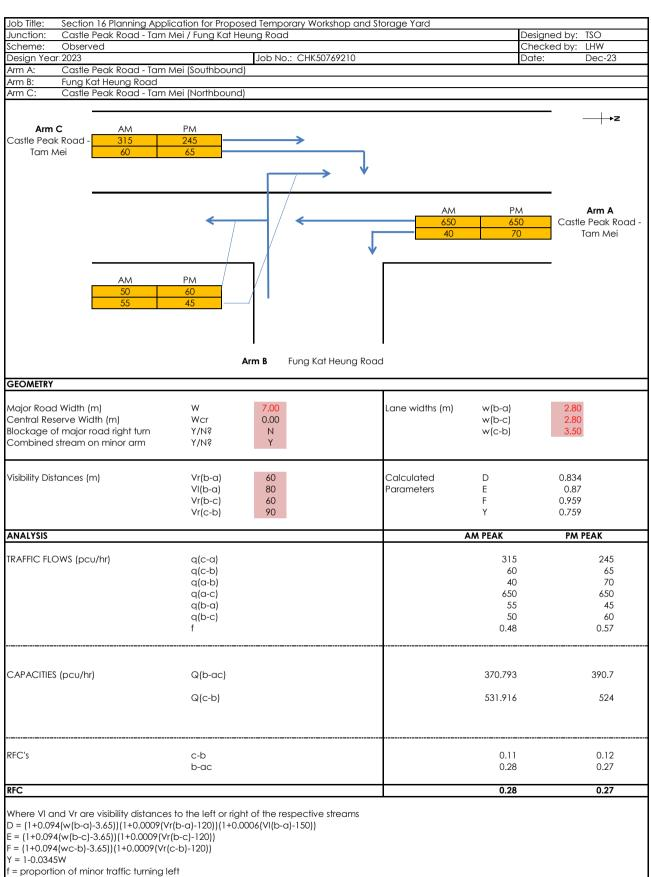
Q(b-a) = Q(b-c)\*Q(b-a)/(1-f)\*Q(b-c)+f\*Q(b-a) Capacity of combined streams
