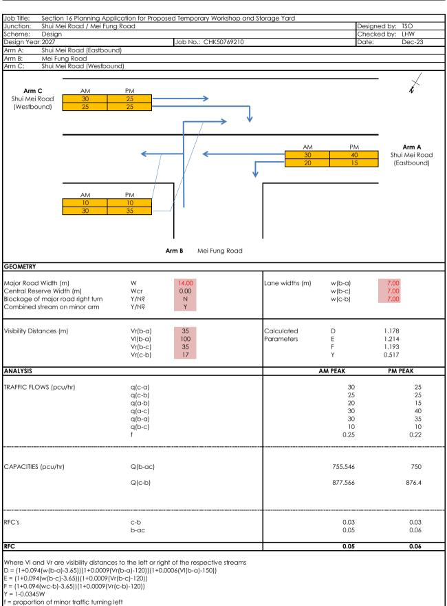
Q(b-ac) = Q(b-c)\*Q(b-a)/(1-f)\*Q(b-c)+f\*Q(b-a) Capacity of combined streams
