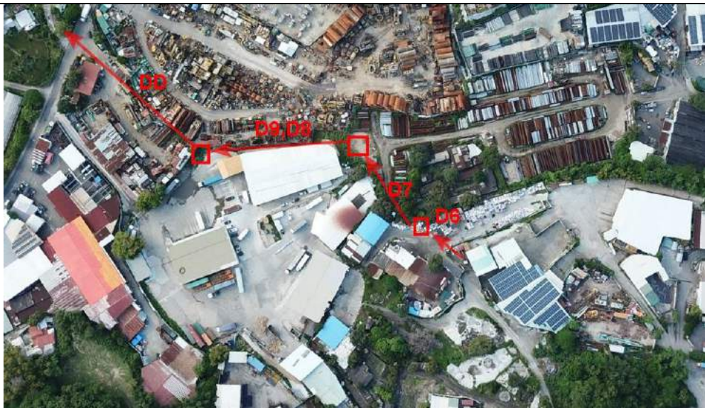
photo of route of D6-D9, to be collected at CP10, discharging to DD
