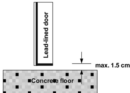
The door and door frame must have the same lead equivalence as the adjacent wall. The protective lead covering the door must overlap that of the door frame by at least 1.5cm. The protective lead covering the door frame must overlap the concrete or brick in the wall by at least the same amount as the thickness of the concrete or brick (Fig 5).
