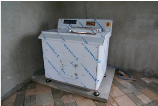
Photo 5: Food waste composting system (Photo credit: Green Power)
