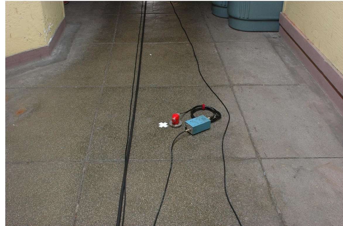
PHOTO 2 GEOPHONE MOUNTED ON THE FLOOR OF THE TSAN YUK HOSPITAL
