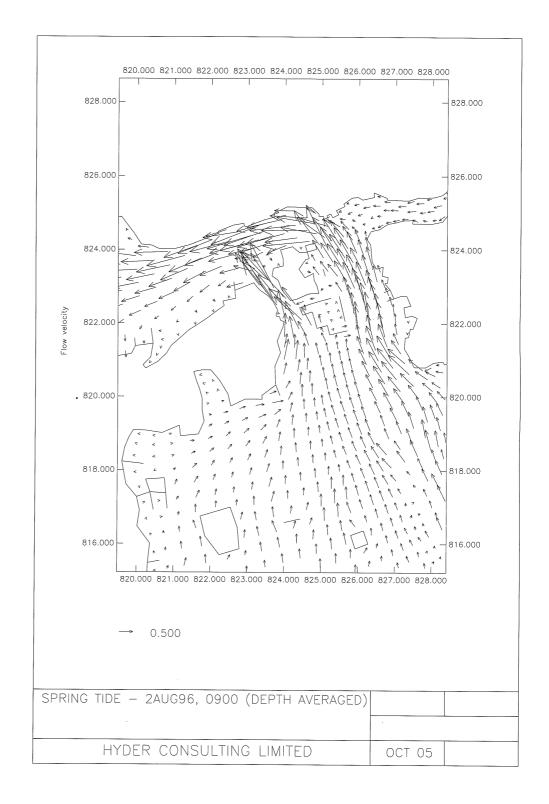
Figure 3-2 Depth Average Peak Velocities during a Typical Flood Tide in a Wet Season
