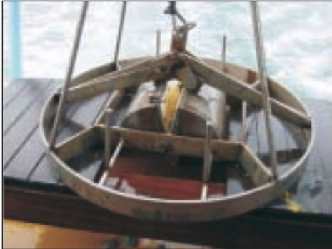
Modified Van Veen grab as used to collect samples at South Soko and along the proposed pipeline route
