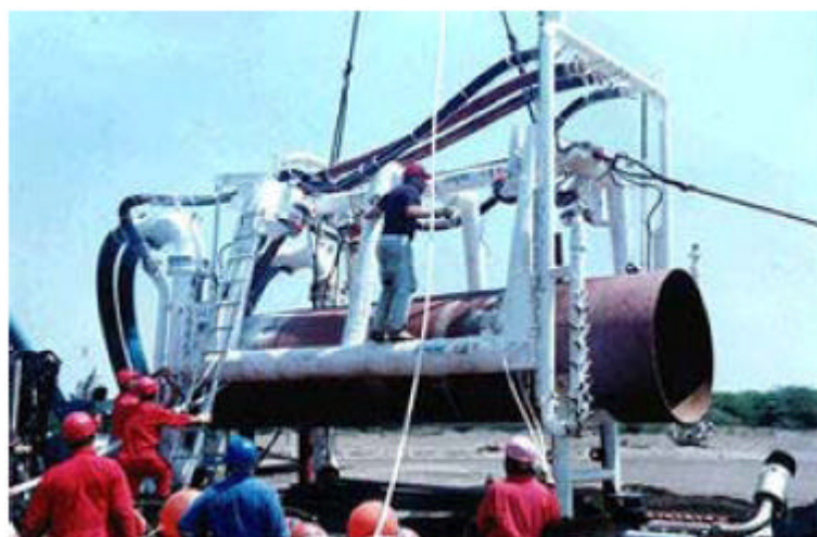
Figure 1.2 “Bengal Tiger” 30 – 60 inch pipeline Jet Sled (OES Equipment)
