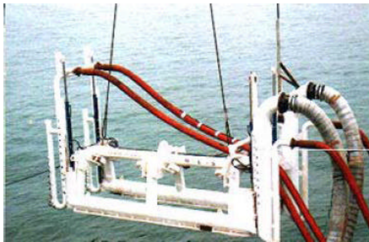
Figure 1.1 “Arabian Leopard” 12 – 30 inch pipeline Jet Sled (OES Equipment)
