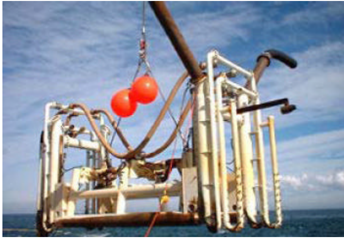
Figure 1.3 “Sumatran Tiger” 20 to 42 inch pipeline Jet Sled (OES Equipment)
