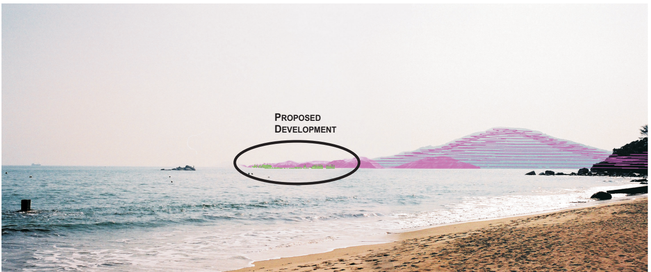
WIREFRAME OF THE PROPOSED DEVELOPMENT AND THE DIGITAL TERRAIN MODEL COMPOSITED ONTO THE PHOTOGRAPH
