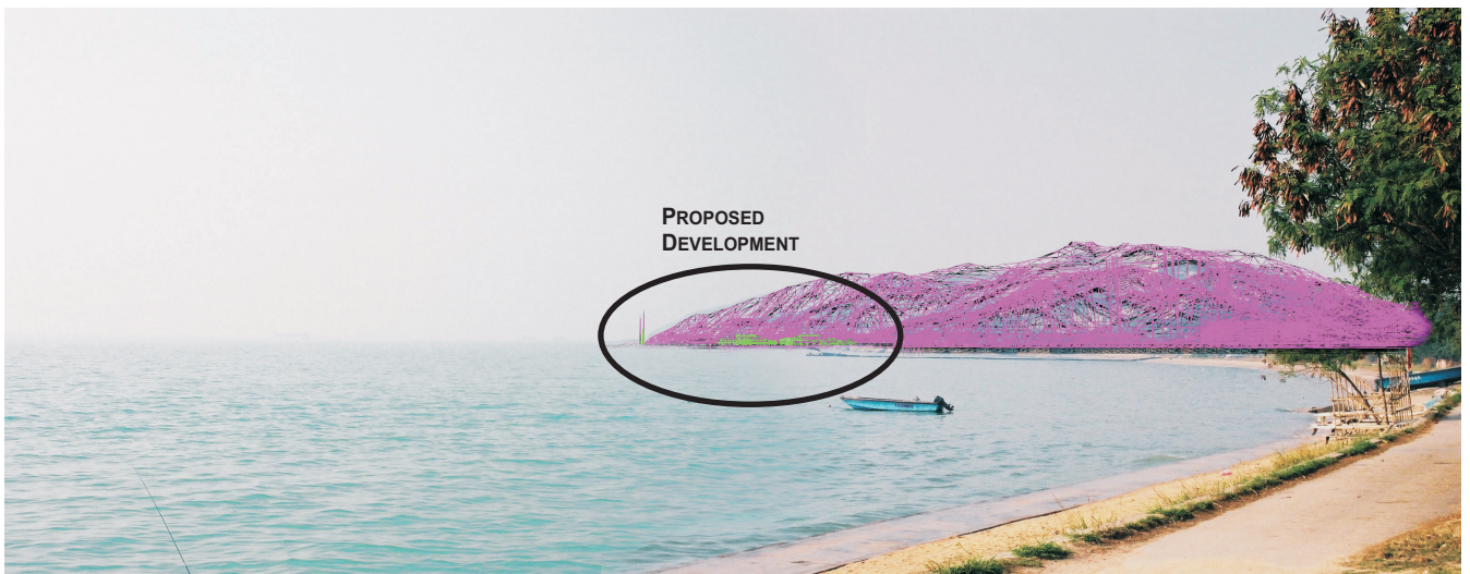
WIREFRAME VIEW OF THE PROPOSED DEVELOPMENT AND THE DIGITAL TERRAIN MODEL COMPOSITED ONTO THE PHOTOGRAPH
