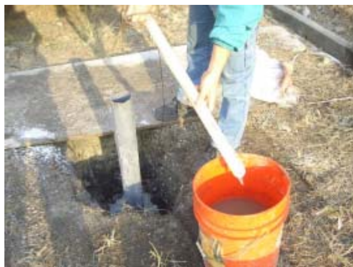
Photo 6 - Well development at location DH8.
