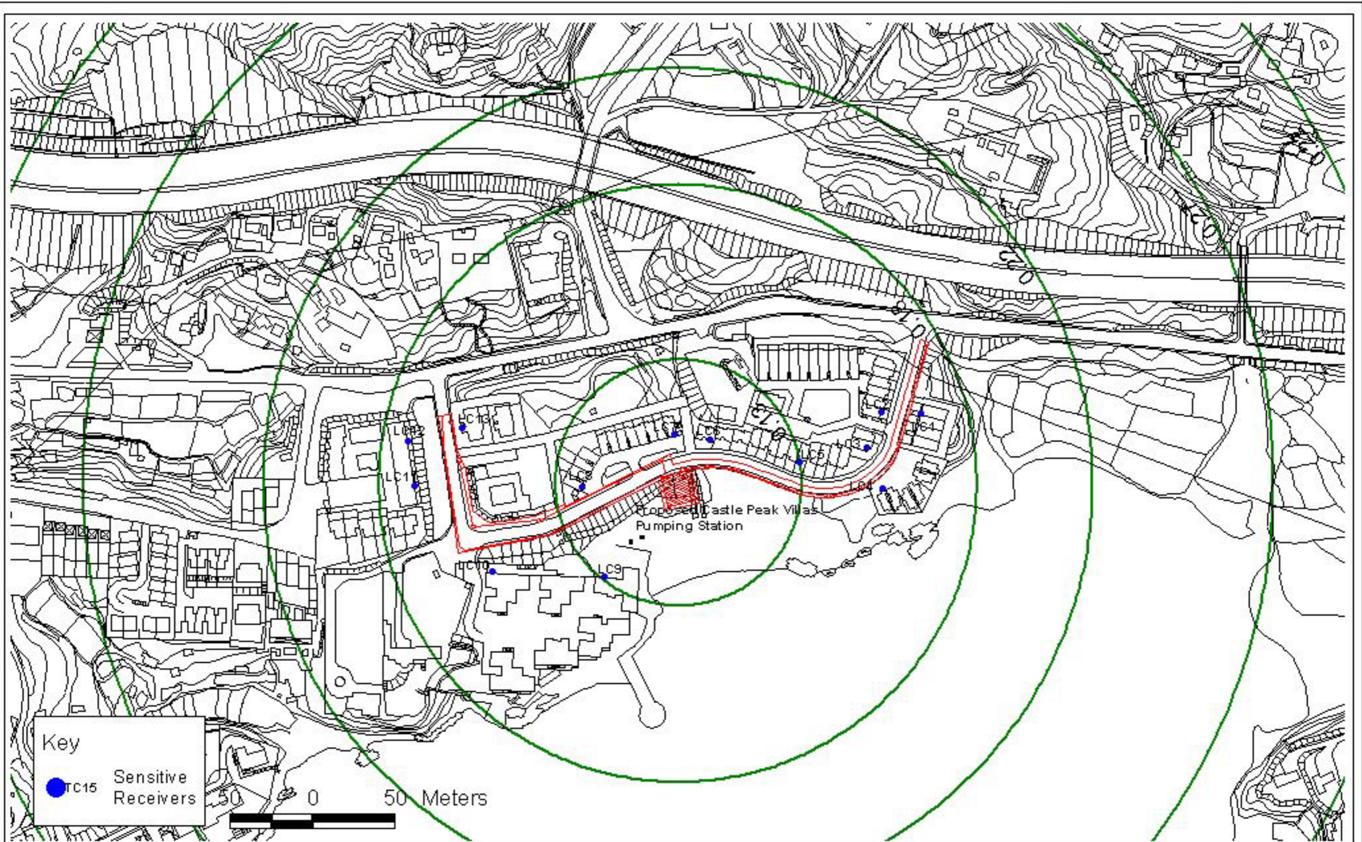
Odour Contour (Unit: ou) Plot at 4.5m Above Local Ground at Stability Class F (Castle Peak Villa Pumping Station)
