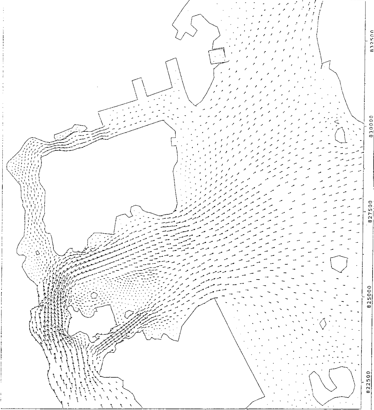
TSUEN WAN BAY FURTHER RECLAMATION, AREA 35 BASELINE, PEAK EBB VECTORS, DRY SEASON NEAP TIDE, SURFACE (LARGE VIEW)
