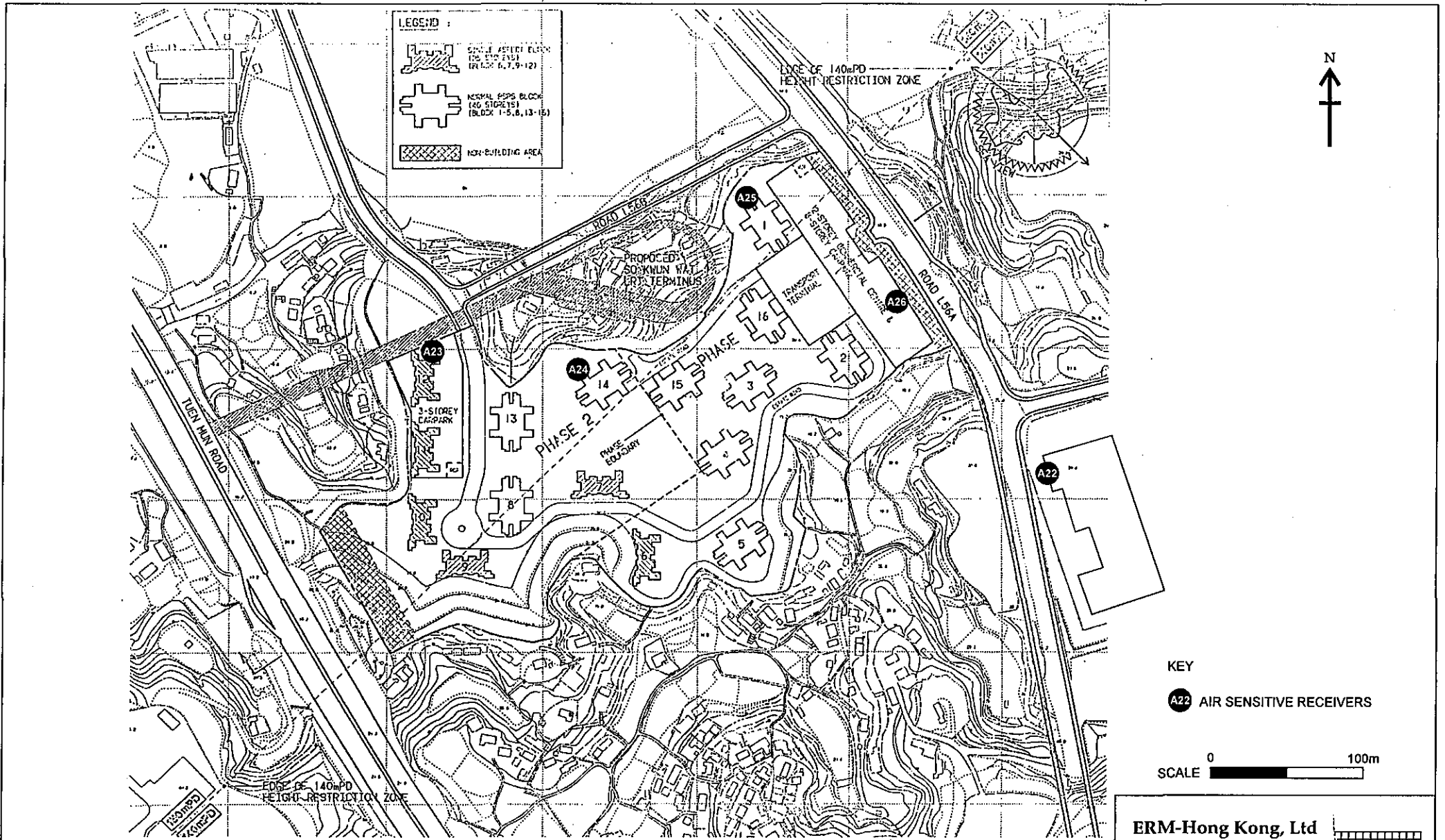
FIGURE 4.4b - LOCATION OF PLANNED AIR SENSITIVE RECEIVERS
