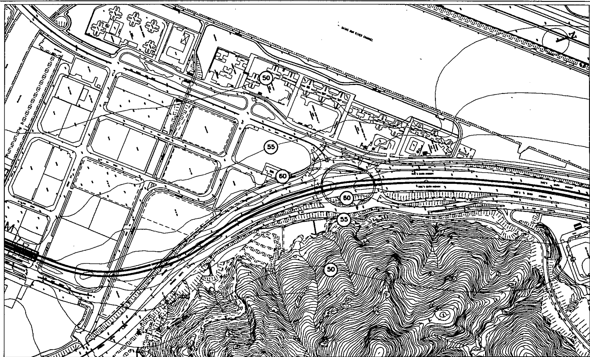
FIGURE 3.5e - Night Time Leq (30 mins) dB(A) Contours (City One Shatin to Shek Mun)
