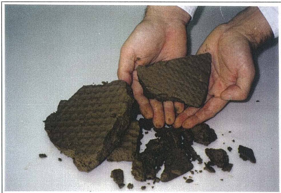
Plate 2.4 WTW Sludge - 30% solids, 70% water from sludge filter press.
