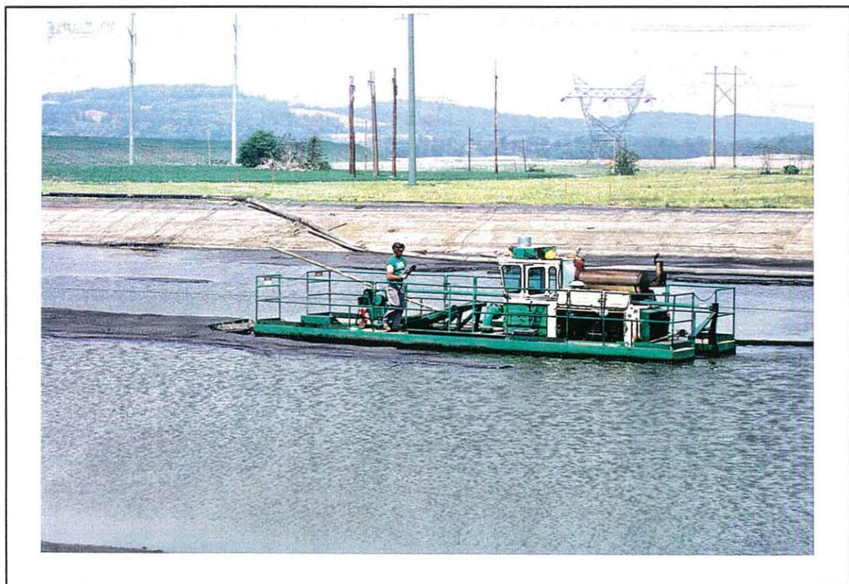
Figure 5.2 Small Dredger working on Ash Lagoon, USA
