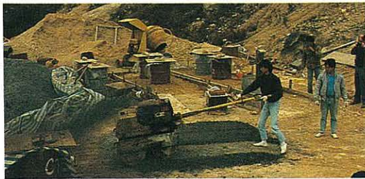
Site trials of PFA/bentonite for use as a refuse tip liner material.
