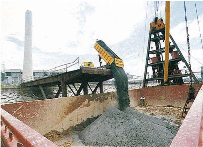
Loading conditioned PFA into a lighter barge. 用輕駁船裝載濕煤灰
