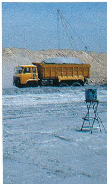
Mobile dust monitoring equipment in use at a PFA fill site.
