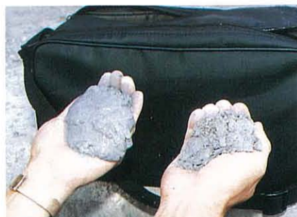
Sample of fill placed below and above water. 於水下、水上的填料樣本
