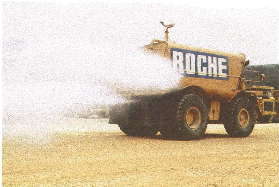
Water Bowser Applying Sea Water for Fugitive Dust Control Exhibit 5.2
