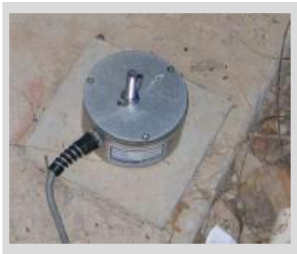
Figure 5.1 – Seismograph for vibration monitoring
