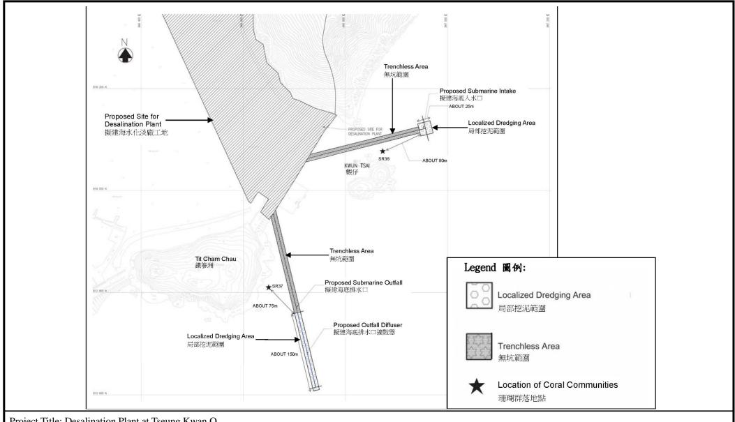
Project Title: Desalination Plant at Tseung Kwan O工程項目名稱:將軍澳海水化淡廠 Dredging Area for the Intake and Outfall Pipe 海底排水及進水口管道的海床挖掘範圍
