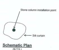
Installed stone columns and barges not shown for clarity.
