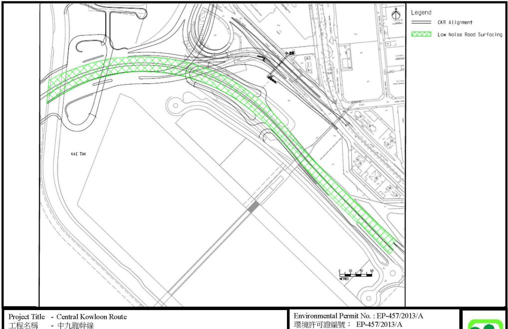
Figure 4d – Location of Noise Mitigation Measures for Road Traffic Noise (East Portion)
