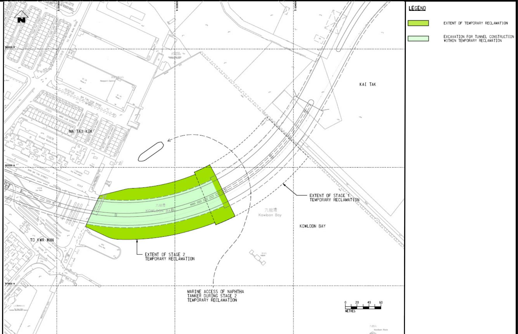
Figure 2b– Proposed Temporary Reclamation and Dredging For Underwater Tunnel (Stage 2)
