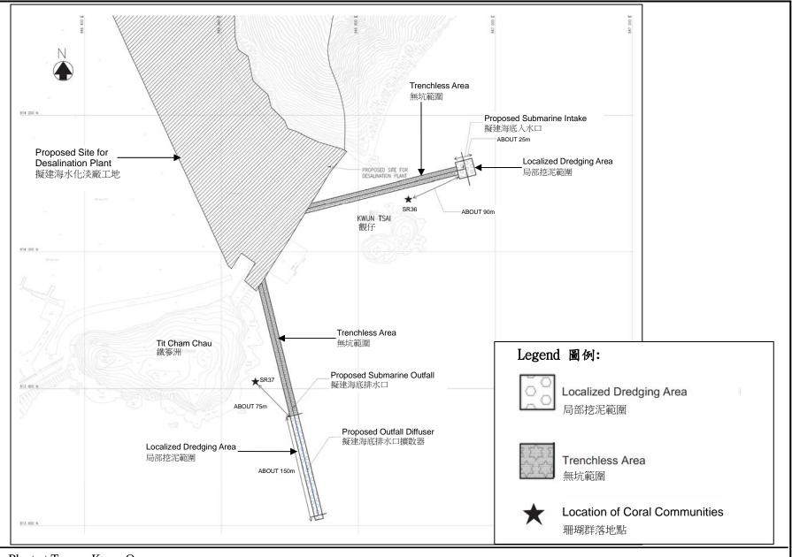
Project Title: Desalination Plant at Tseung Kwan O 工程項目名稱:將軍澳海水化淡廠 Dredging Area for the Intake and Outfall Pipe 海底排水及進水口管道的海床挖掘範圍
