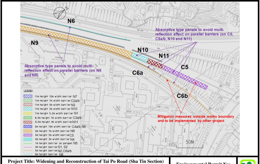
**Figure 2d: Locations of Noise Mitigation Measures (4 of 4)** (Extracted from Figure 2.1d of Environmental Permit Application No.: AEP-463/2013)
