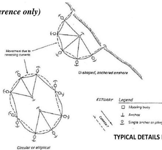
TYPICAL DETAILS FOR FLOATING TYPE SILT CURTAIN DEPLOYMENT
