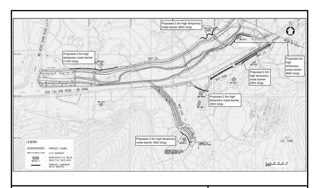
Figure 6 圖六 Locations of Temporary Noise Barrier – Man Uk Pin (MUP03, MUP04A, MUP04B & MUP05) (Sheet 2 of 2)
