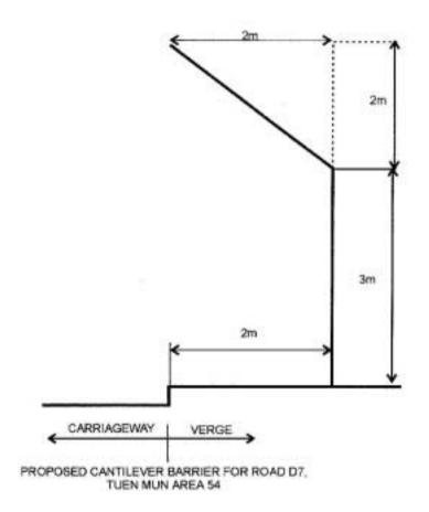
Note :that the dimensions of the noise barriers proposed in this assessment are subject to detailed design when suitable equivalent configurations may be considered to be more appropriate
