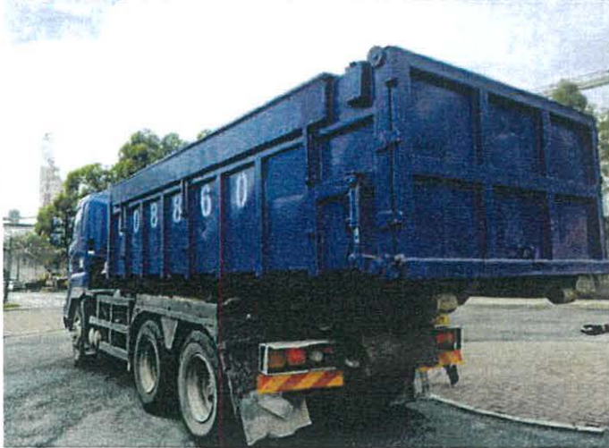
Photo 1 – Enclosed and Water-tight Container Truck for GTW Sludge Transportation
