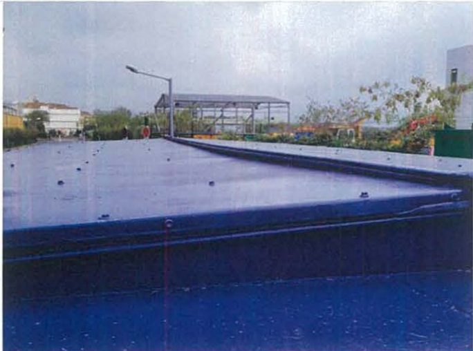
Photo 3 – Top Cover of Enclosed and Water-tight Container Truck
