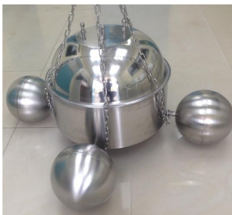
Figure 3: Dynamic Flux hood used for Odour sampling (Covering Area: 0.155m 2 )
