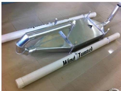
Figure 1: Wind Tunnel used for Odour sampling (Covering Area: 0.384m 2 )
