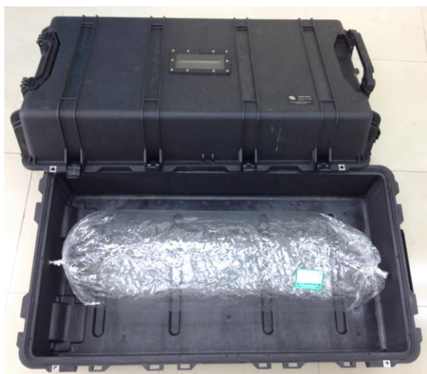
Figure 2a: Sampling Bag & Air-tightened Sampler
