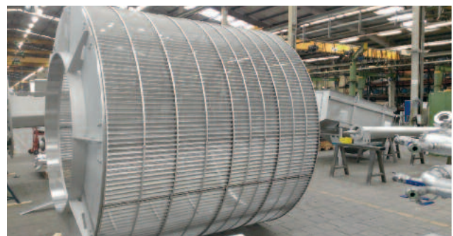
ROTAMAT® STAR screen basket, 2600 mm diameter, 1 mm perforation, acid-treated in a pickling bath and passivated
