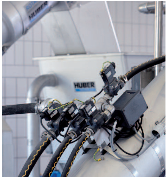
HUBER Rotary Drum Fine Screen ROTAMAT® with integrated screenings washing IRGA
