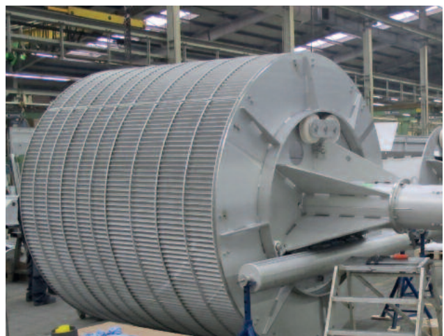
HUBER Perforated Plate Screen ROTAMAT® STAR, 2600 mm diameter, 1 mm perforation
