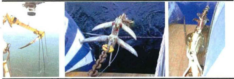
Figure 2.2 Typical grapnels used to penetrate seabed, grip, cut and recover cable
