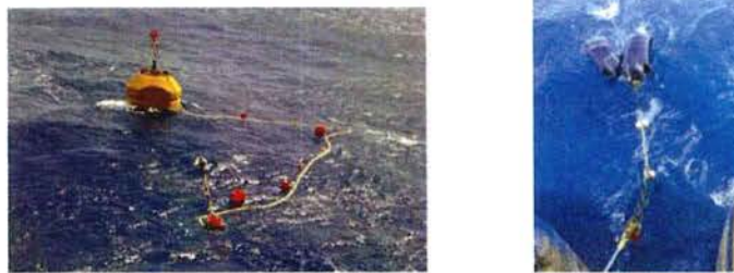
Figure 2.3 Typical buoy types used for connecting to cable end by rope
