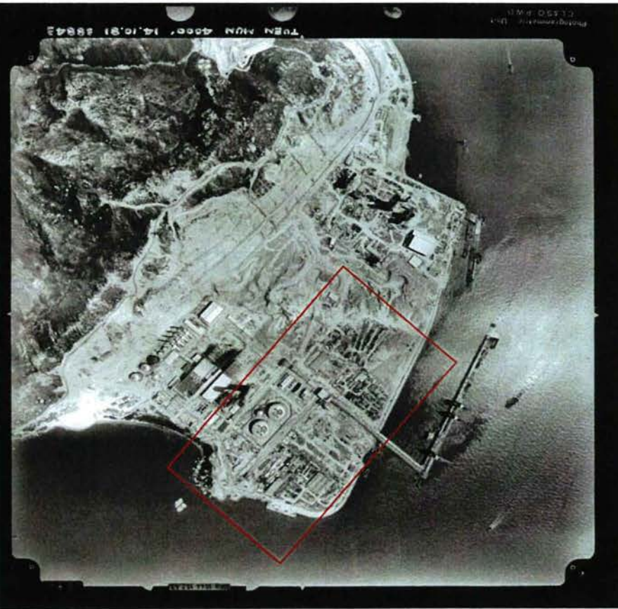
Year 1981 (ref: 38843, height: 4,000ft) – Reclamation is completed and the power plant was under construction. Some temporary structures were observed in the construction site.
