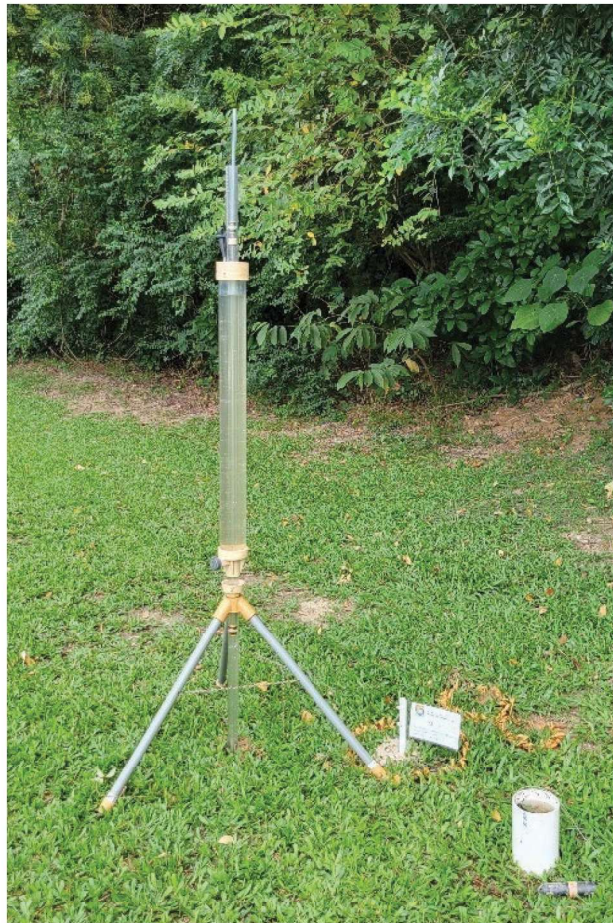
Figure 7F – In-situ measurement of the saturated hydraulic conductivity of the top-layer soils using a Geulph permeameter.
