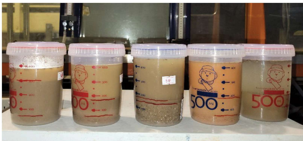
Figure 7G – Mason Jar Soil Test to determine the soil type
