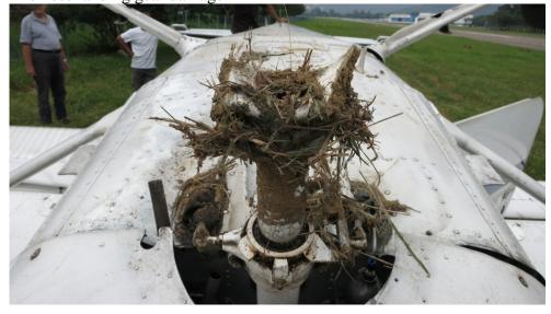
The nose landing gear damage
