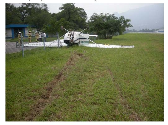
The markings on ground – front wheel and right main wheel
