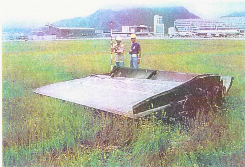
Figure 15. Right Inboard Flap from Ship 518 (China Airlines)
