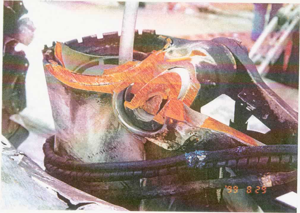
Fractured Center Landing Gear Oleo (Figure 13)
