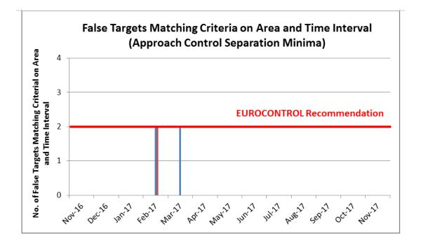
For Approach Control airspace, false target reports (as shown by the bars) did not exceed the figures specified in the EUROCONTROL Specification.
