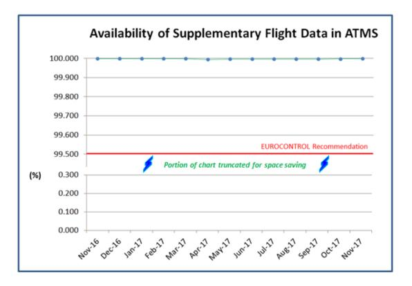
The availability of supplementary flight data (as shown by the dotted line) has exceeded the requirement of 99.5% specified in the EUROCONTROL Specification at all times.
