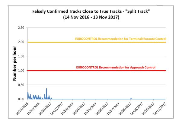
Falsely confirmed track cases per hour (as shown by the waves at bottom left) were less than the figures specified in the EUROCONTROL Specification.
