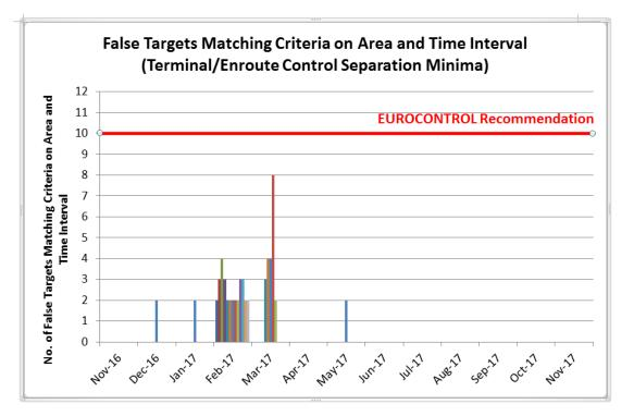
For Terminal/Enroute Control airspace, false target reports (as shown by the bars) were less than the figures specified in the EUROCONTROL Specification.
