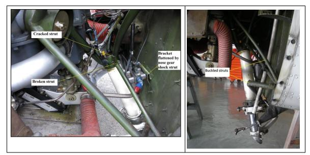
Figure 6a Damaged engine mount truss
