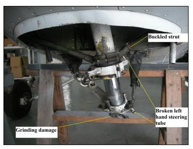
Figure 5 Damage of nose landing gear
