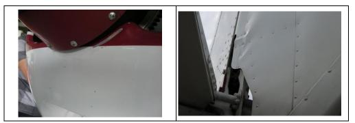
Figure 10 Rub mark on engine cowling
