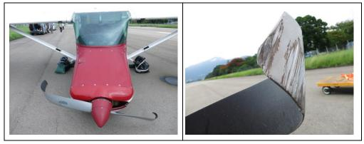
Figure 8 Propeller blades bent rearward
