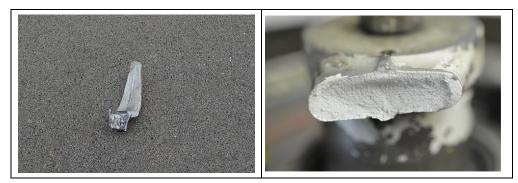
Figure 3 Broken nose wheel fork
