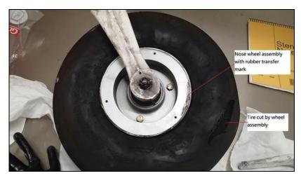
Figure 2 Damage on nose wheel assembly
