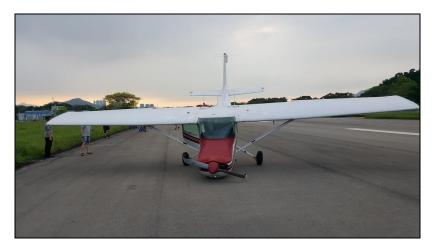
Figure 1 Aircraft stopped in a nose down position on Runway 11
