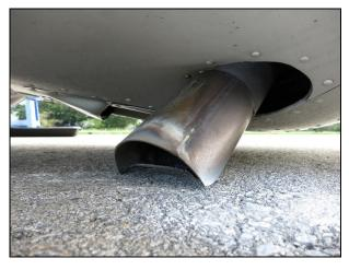
Figure 7 Grinding damage of exhaust pipe
