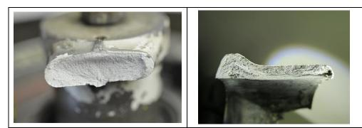
Figure 15 Broken nose gear fork at axle
