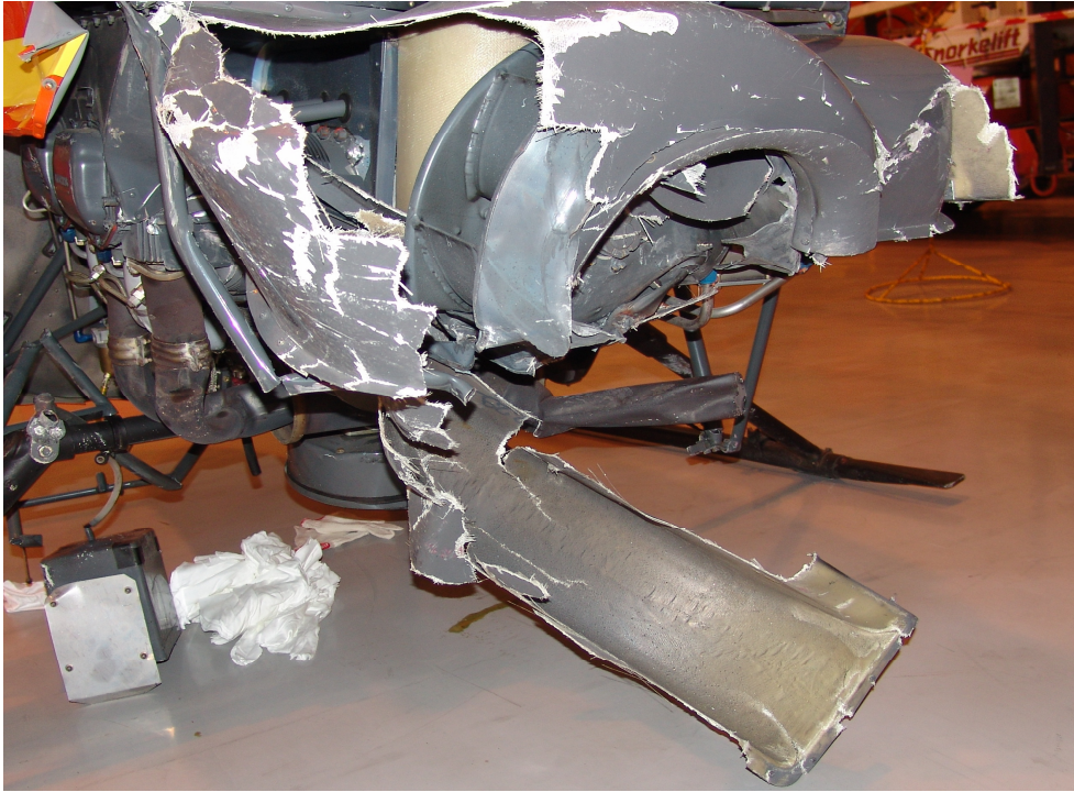
Photograph 8 The Centrifugal Cooling Scroll and Fanwheel
