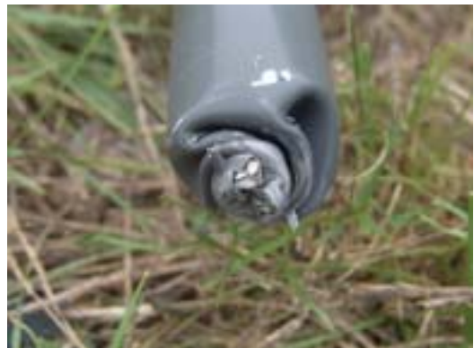
Photograph 6b The Other Broken End of Tail Rotor Drive Shaft
