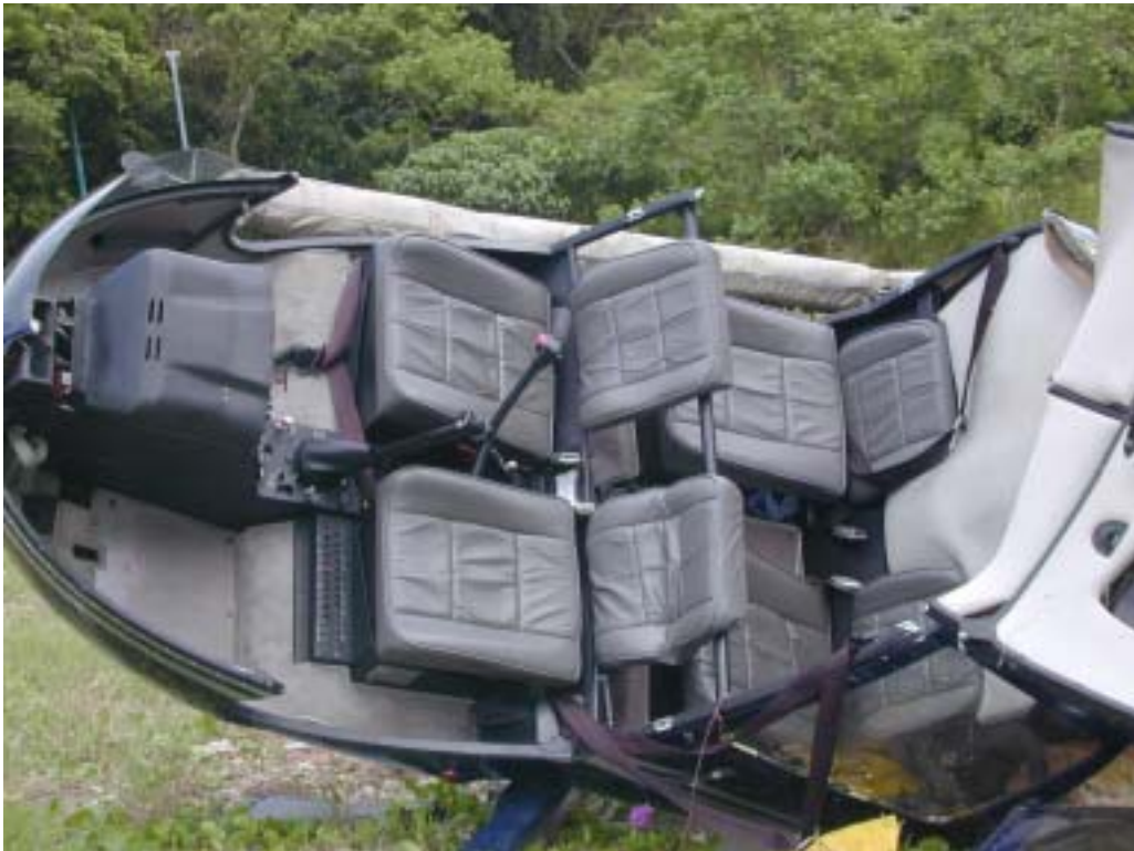
Helicopter Cabin (perspex canopy removed by emergency service personnel during rescue operation)
