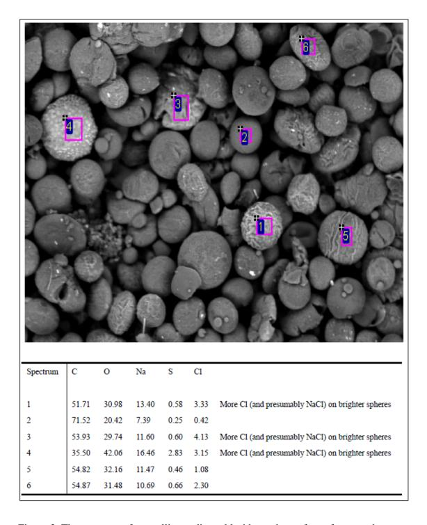
Figure 3: The presence of crystalline sodium chloride on the surface of some spheres.
