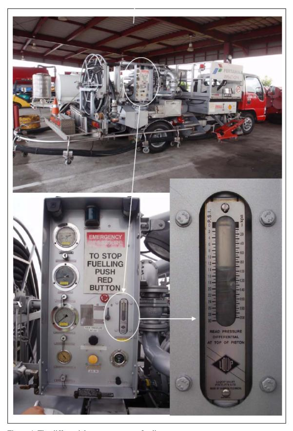
Figure 4: The differential pressure gauge of a dispenser.
