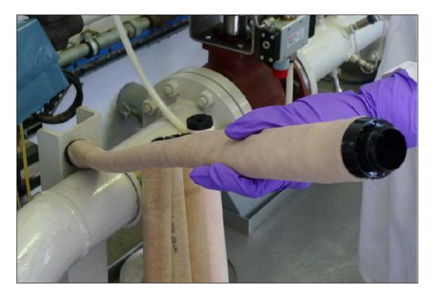
Figure 5a: A collapsed monitor losses the structural rigidity.
