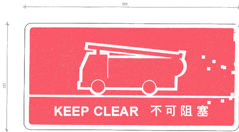
EMERGENCY VEHICULAR ACCESS ROUTE SIGN ALONG EVA NOT IN THE FORM OF CARRIAGEWAY
