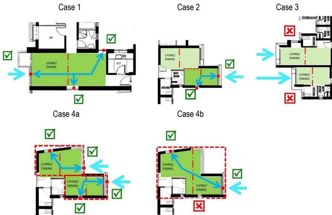
Figure 15 Openable Windows Located at Different Halves of Habitable Spaces
